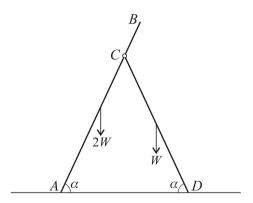
The diagram shows a pair of stepladders modelled by two uniform rods, AB of length 5a and weight 2W and CD of length 4a and weight W, smoothly hinged at C. The stepladders rest on a rough horizontal floor with A fixed so that it cannot slide. The angles CAD and CDA are both equal to  $\alpha$ . By taking moments about A for the system, find the normal contact force at D.
