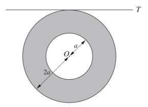
A uniform lamina of mass m is bounded by concentric circles with centre O and radii a and 2a. The lamina is free to rotate about a fixed smooth horizontal axis T which is tangential to the outer rim (see diagram). Show that the moment of inertia of the lamina about T is  $\frac{21}{4}ma^2$ . [5]
