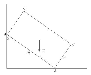
The diagram shows a cross-section ABCD of a uniform rectangular block of weight W. The lengths of AB and BC are 2a and a respectively. The edge through A rests against a smooth vertical wall and the edge through B rests on a rough horizontal floor. The coefficient of friction between the block and the floor is  $\mu$ . The block is in equilibrium with AB inclined at an angle  $\alpha$  to the vertical. Show that the wall exerts a force of magnitude  $\frac{1}{4}(2\tan\alpha - 1)W$  on the block.
