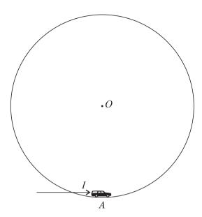
The diagram shows a toy car of mass m which can move freely on a circular track of radius a and centre O. The track is fixed with its plane vertical. The car is given a horizontal impulse of magnitude I when it is at rest at the lowest point A of the track. The car may be modelled as a particle moving without resistance. Show that the force that the track exerts on the car when the radius to the car makes an angle  $\theta$  with OA has magnitude
