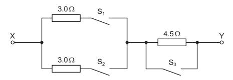
Which switch positions give a resistance of  $6.0 \Omega$  between X and Y?
