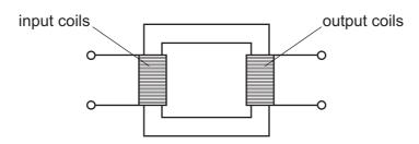
The output voltage needs to be lower than the input voltage.
