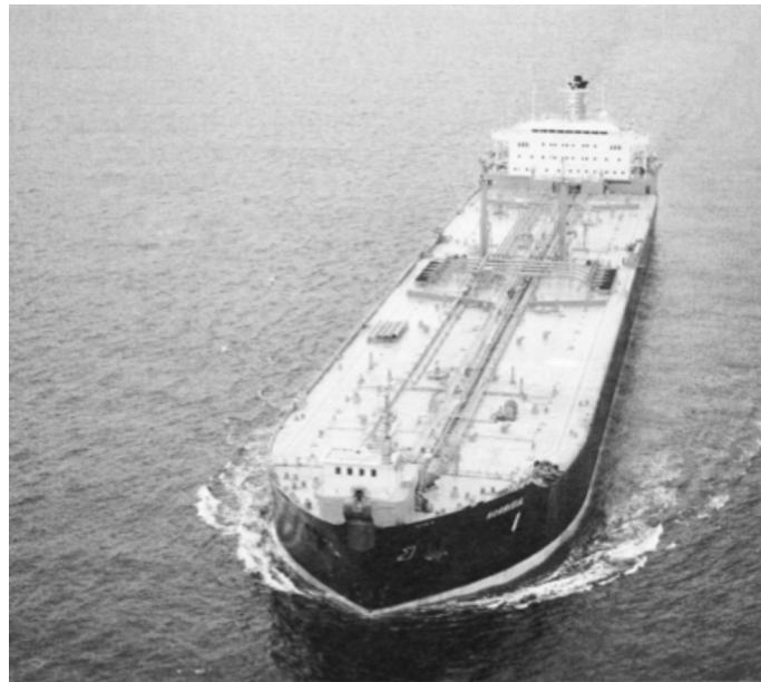
Fig. E1.4 The oil tanker Norrisia has a total mass of approximately 150 000 tonnes when fully laden. It therefore needs to displace 150 000 tonnes of water in order to float.
